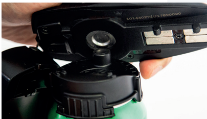
1. Place the Detaching Well of the Detacher onto the Knob of the Can Guard
